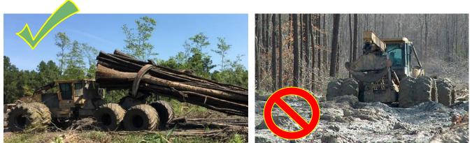
Skidders should only run on the shovel trail (left), and not directly on the bare ground of the swamp (right).
